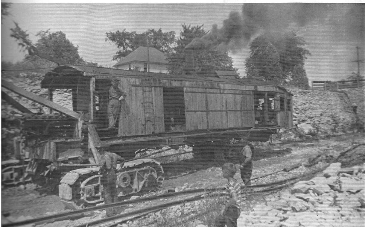
Steam shovel "39" was used in Kelleys Island Lime and Transport Co. This quarry stopped operation in 1940.
